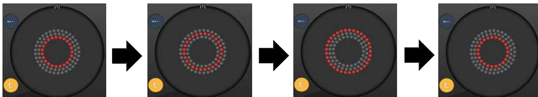
System Automatically Advances to Next Ring when Auto Advance Feature is Enabled
